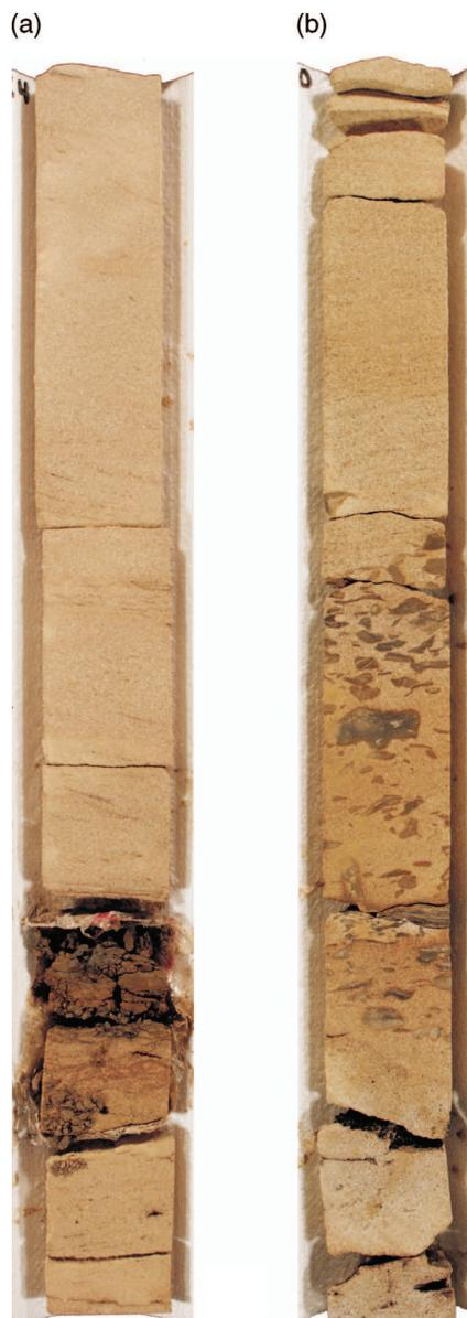
**Figure 5** Representative core examples of the main lithologies at Corbula Gulch: (a) is between 7.3 and 7.9 m depth in hole 4 and shows cross-bedded sands and a clay drape within CD2; (b) is between 15.2 and 15.8 m depth in hole 5 and shows mudstone interclast conglomerate in CD1, just above the basal flood-plain mudstone. The diameter of the core is  $\sim 6.3$  cm (2.5 inches).
